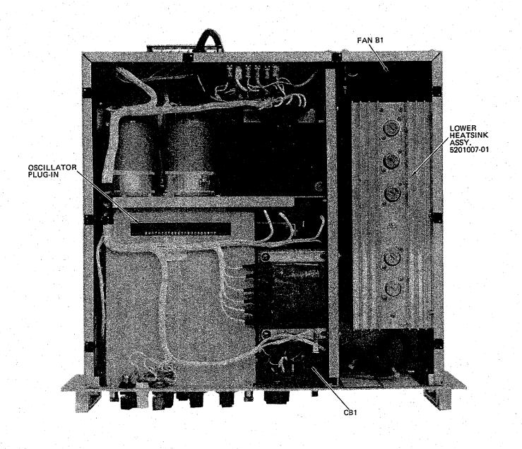
Figure 5-2. Model 251B Bottom View.
