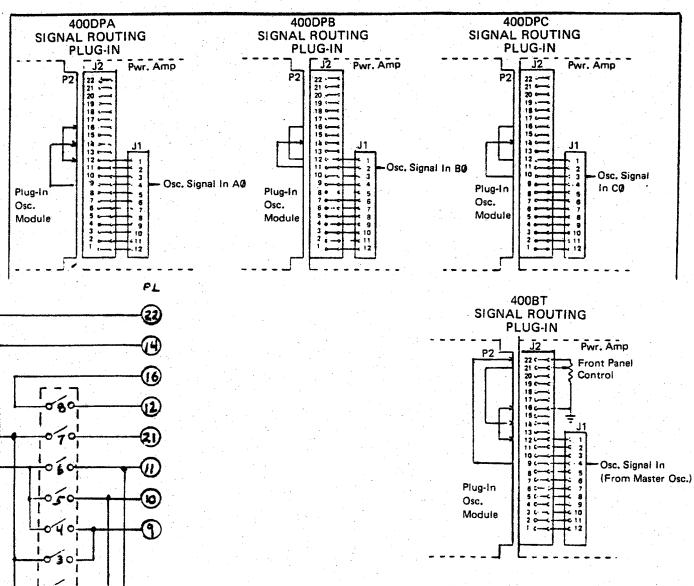
Figure 4-5. Signal Routing Plug-In Connections
