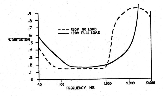
Figure 1-2. Typical Harmonic Distortion at Rated Power
