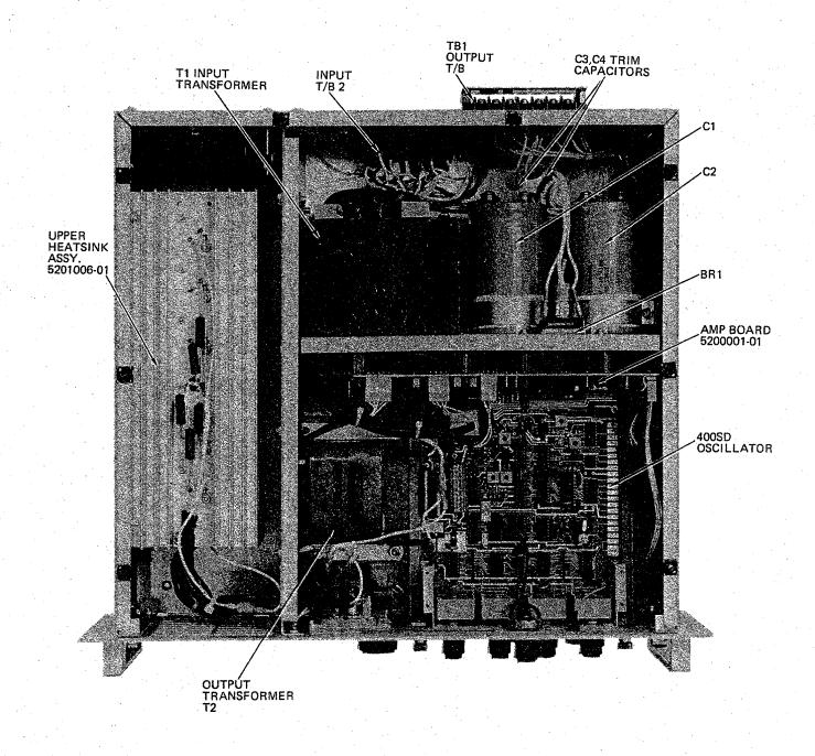
Figure 5-1. Model 251B Top View
