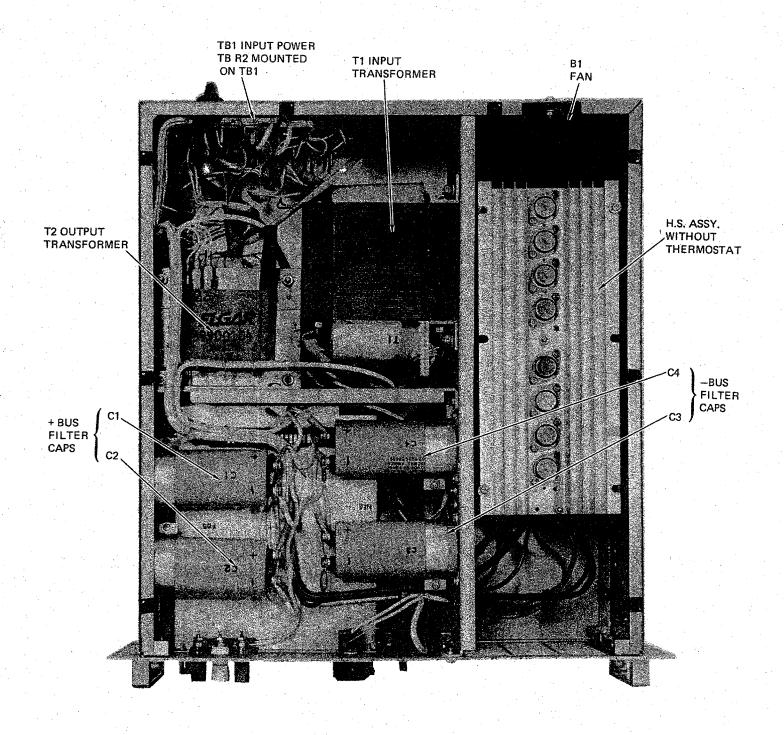
Figure 5-3. Model 501B Top View
