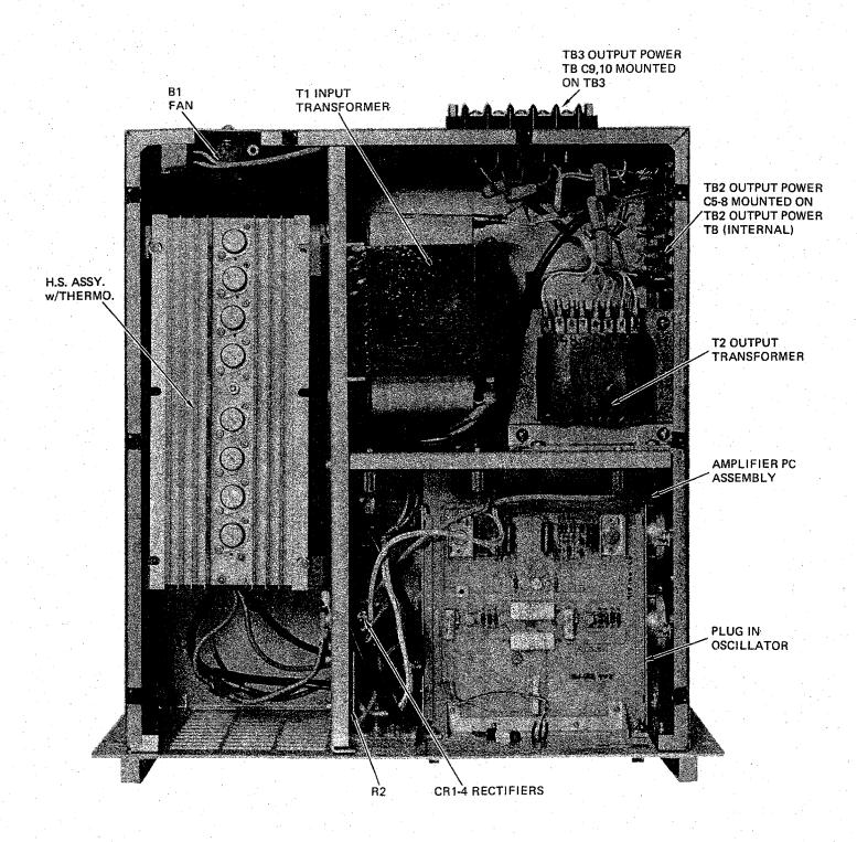
Figure 5-4. Model 501B Bottom View
